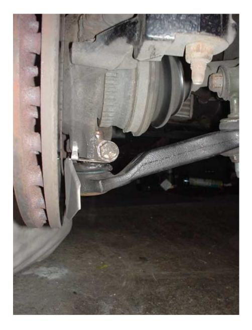
Wishbone balljoint and brake disc splash guard can be seen.
