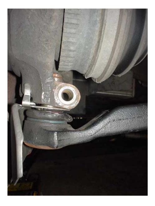
Wishbone balljoint nut and bolt removed (both 17mm) you may need to tap out the bolt.
