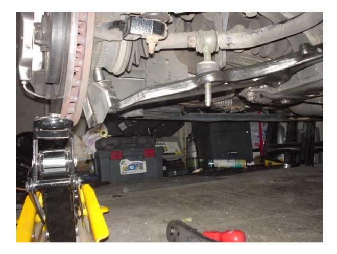
Wiggle the new wishbone in place, it can be easier if you do this with the drop link completely removed. Don't worry about lining up the balljoint for now just concentrate on getting the 4 bolts into place, just nip them us loosly for now. When this is done refit the drop link and push down on the wishbone end until it's far enough down to locate the drop link in it's hole (don't forget the upper bush and washer).
