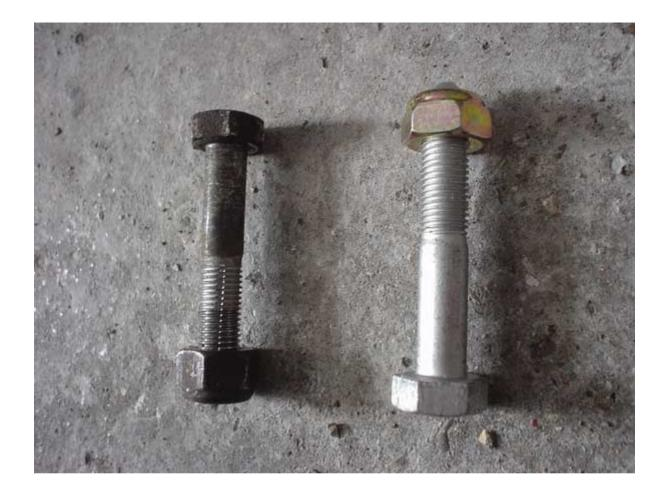
A shot of the wishbone balljoint securing nut and bolts. I used new ones as the threads were damaged taking them out and the new nut is a nylock style self locking nut.
