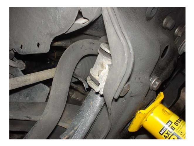
Next, jack and support your car, I used this spot as it's steady and away from the wishbone mounting bolts. You can use the normal jacking points if you prefer. You'll need an axle stand as the jack is used later.
