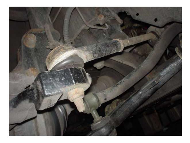
Just a shot of the track rod end, John, mark or count the number of exposed threads, then slacken the securing nut fully and take off the balljoint nut. Split the balljoint and just unscrew it from the steering arm. Put the new one on the same amount of threads and get the tracking checked when you're all done. Nut torque is 34NM
