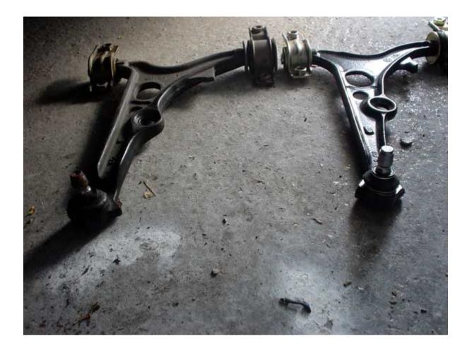
Next, slacken the 17mm nut holding the drop link to the end of the anti-roll bar and remove the 4 15mm bolts holding the wishbone to the subframe. Be carefull with these as there are 3 different lengths and the **must** go back in the same holes. Jack up the brake disc as high as possible and simple yank the wishbone out! This photo shows the old and new wishbones side by side.
