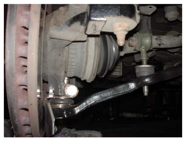
Finally, push down on the wishbone end again and manouvre the balljoint into it's home on the stub axle (you need to push down quite hard on the wishbone but it is possible).
