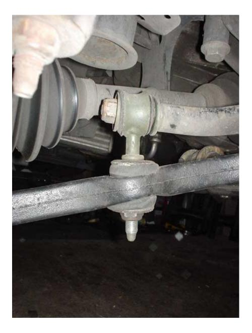
This is the drop link which attaches the end of the anti-roll bar to the wishbone. With the wheels on the ground remove the lower nut and take off the bush and washer (17mm)
