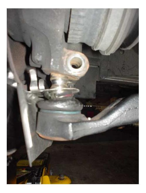
Wishbone balljoint split from stub axle. It may make it easier if you jack up the bottom of the brake disc and push down on the wishbone. Keep the car in gear to do this else the disc will just spin. Mine had a split rubber boot but these can be bought seperately if that's all that's wrong.
