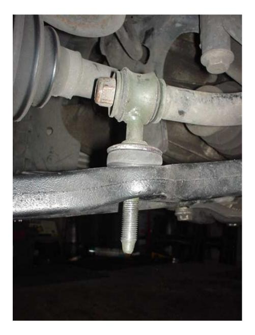
Drop link with securing nut and bushes removed.
